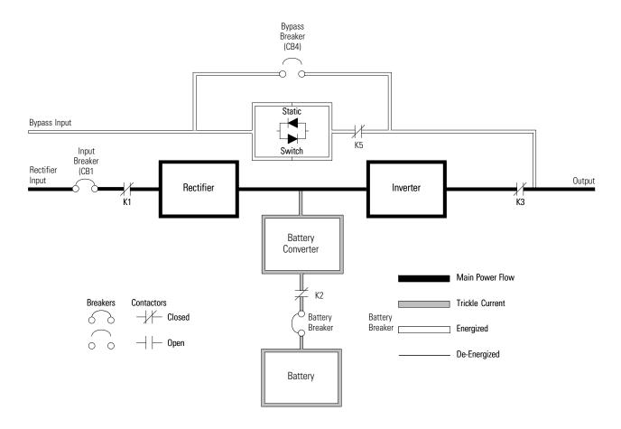
**NOTE** On an UPS configured as an IOM, the bypass input, static switch, bypass breaker (CB4), and K5 are not present.
